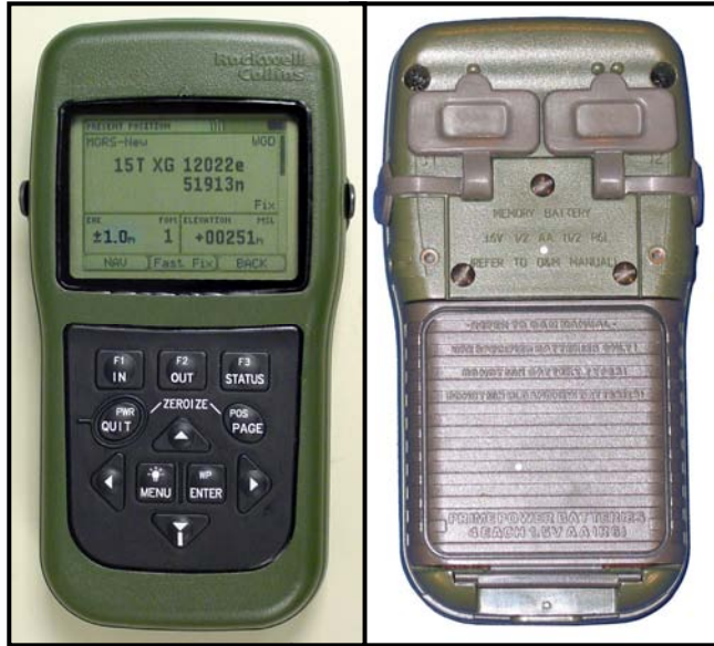
Figure K-1. Defense advanced GPS receiver (DAGR).
