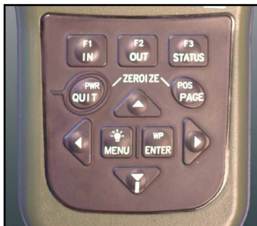
Figure K-2. Function keys.
